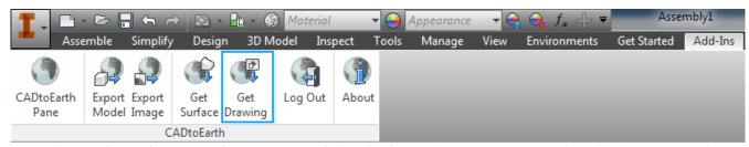
Another unique feature of CADtoEarth is ability to import curves sketched on Google Maps into the CAD environment. In order to do so the Get Drawing command should be launched from the CADtoEarth toolbar.
