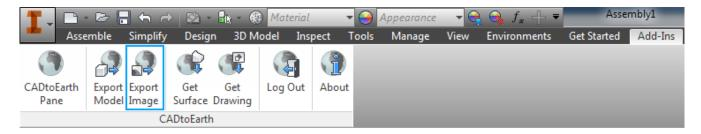
The Export Image command should be used to save the current model view as an image and upload it to the CADtoEarth cloud service where it can be placed onto the Google Maps. Once the command is launched the Save As dialog would appear:
