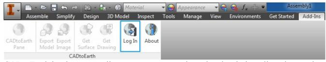
CADtoEarth implements a client-server system, where the plug-in is a client that sends a request to the server that returns a response. To communicate, you will need to login to the plug-in with your account credentials.
