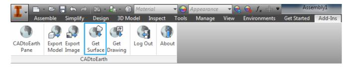
One of the unique features of CADtoEarth is the ability to import certain part of the Earth surface into the CAD application. In order to do this the Get Surface command should be launched from the CADtoEarth toolbar.
