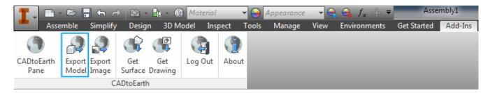
The Export Model command should be used to export the model currently opened model in Autodesk Inventor to Google Earth and upload the resulting file to the CADtoEarth cloud service. Once the command is launched a form with several options appears:
