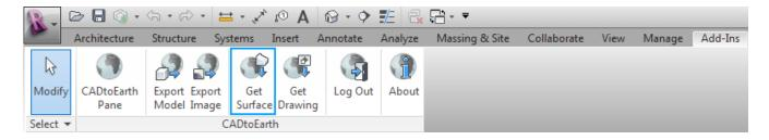
One of the unique features of CADtoEarth is the ability to import certain part of the Earth surface into CAD application. In order to do this the Get Surface command should be launched from the CADtoEarth toolbar.
