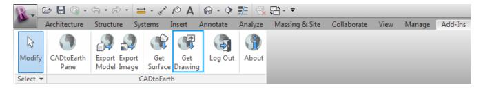
Another unique feature of CADtoEarth is ability to import curves sketched on Google Maps into the CAD environment. In order to do so the Get Drawing command should be launched from the CADtoEarth toolbar.
